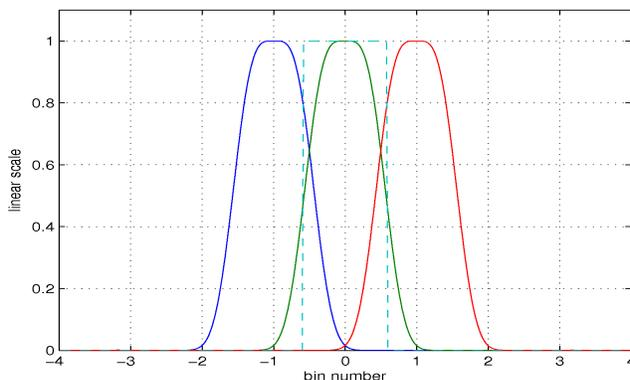
*Frequency response of the optimized FFT signal processing pipeline. The dashed lines illustrates the equivalent noise bandwidth (ENBW) for the corresponding spectral bin.*
